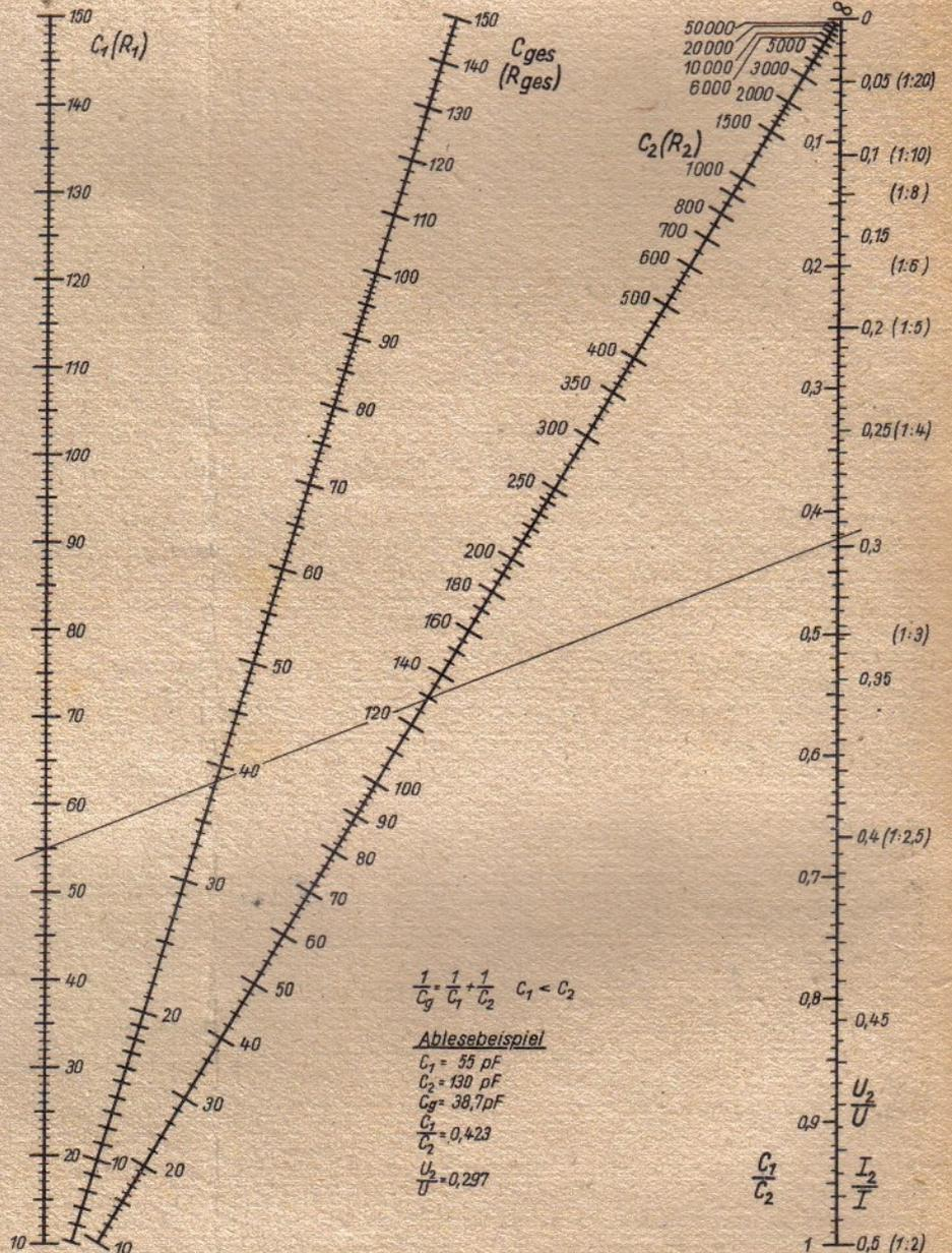
$$\frac{1}{C_g} = \frac{1}{C_1} + \frac{1}{C_2} \quad C_1 < C_2$$
